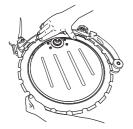
Fit the support roller guard and ensure that the flanges on the guide rollers still enter the blade's grooves correctly. Now tighten the three screws fully.
